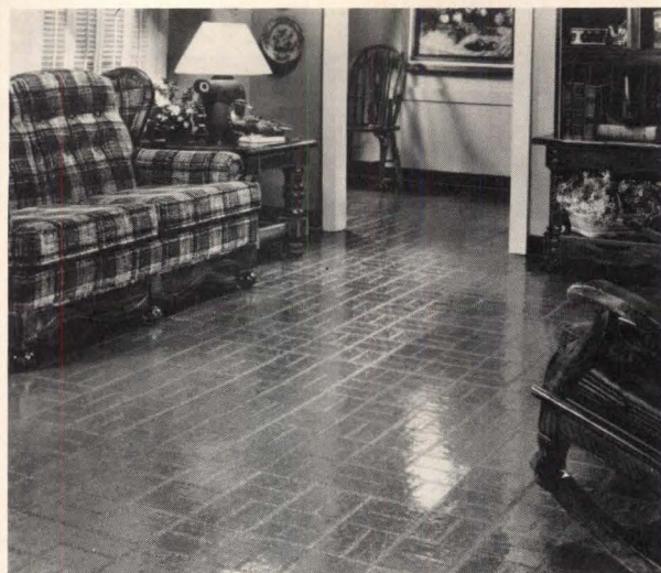
No-wax vinyl asbestos tile, "Glazed Brick" (above), comes in red or white in 12" squares. The tile surface is slightly dimpled. Azrock, San Antonio, TX. Circle 205 on reader service card
