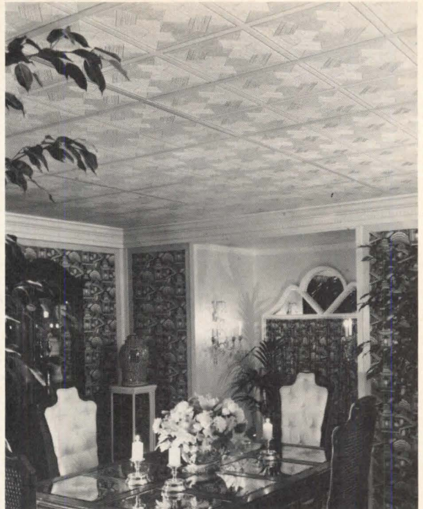
Suspended ceiling panels (above) simulate inlaid wood. The 2'×4' panels may be installed using a "Super White Grid," which is color coordinated to match panel grout lines. Armstrong, Lancaster, PA. Circle 237 on reader service card
