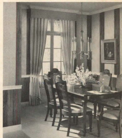
"Woodpaper" paneling —plywood overlaid with wallpaper—comes in a variety of patterns. Designs shown: a geometric print (above chair-rail) and a woodgrain print (below chair-rail). Plywood Panels, Norfolk, VA. Circle 259 on reader service card
