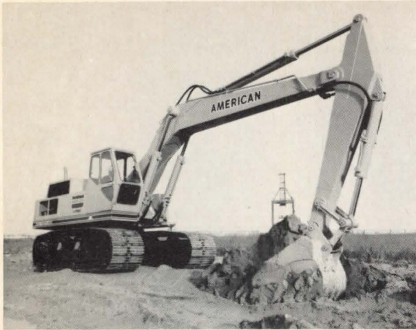
Hydraulic backhoe (above), powered by a 300-hp engine, has a weight of 316 lbs per hp. Standard digging depth is 304 13 / 16 "', but can be extended to 352 13 / 16 "' with a longer, optional arm. American Hoist & Derrick. Circle 244 on reader service card
