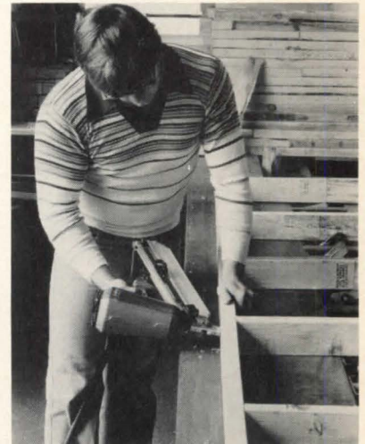
Pneumatic nailer (above)—designed for use in manufactured-housing production plants—is suitable for trussing, framing and sheathing. Compact tool is 16 1/8" long x 12 1/8" high. Duo-Fast. Circle 260 on reader service card
