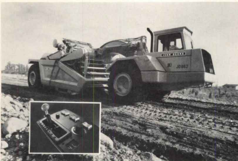
Elevating scraper (above) features an automatic transmission that is controlled by a microprocessor. A digital readout display (see inset) tells the operator what gear he is in, when the torque converter lockup clutch is engaged, or if any electrical problems exist. John Deere. Circle 257 on reader service card
