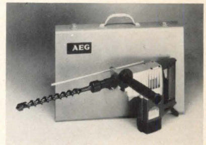
Electro-pneumatic rotary hammer , "Model PH 240 D" (above), is designed for high-speed drilling into concrete. The tool can handle solid bits up to 1", core cutters up to 2 1/2" and self-drilling anchors up to 1/2". UL-listed tool weighs 11 1/2 lbs. AEG. Circle 259 on reader service card
