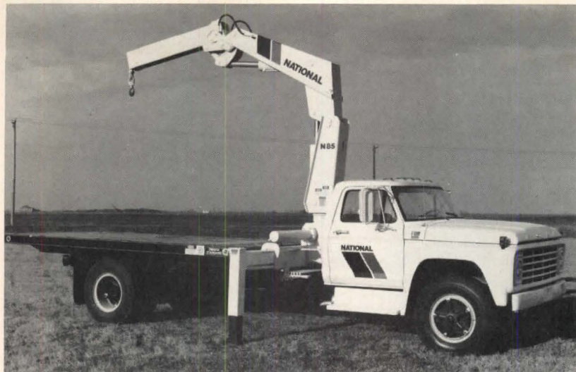
Truck-mounted articulating crane , "Model N-85" (above), can reach 34' above and 20' below the truck frame. Lifting capacity is 14,400 lbs. Accessories include a pallet fork, clam bucket and grapples, a winch and a hydraulic auger. National Crane. Circle 254 on reader service card
