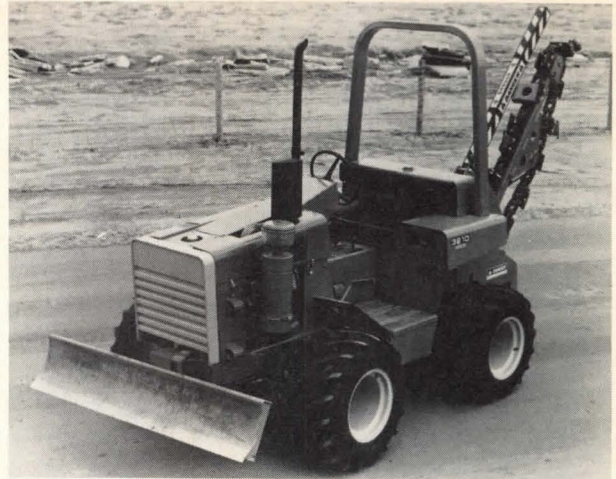
"Modularmatic" vehicle (above) is a basic unit that can be equipped with modules for trenching, plowing, backhoe work or restoration. Machine is powered by a 30-hp engine. Ditch Witch. Circle 248 on reader service card
