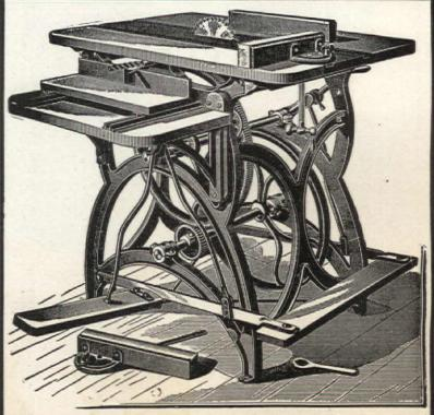
Center part of top is made of fron frame, 30 inches high. Center part of top is made of fron accurately planed with grooves on each side of saw gauges to slide with grooves on each side of saw for gauges to slide in. Steel shafts and best babbitt metal boxes. Gears are all machine cut from solid fron. Boring table and side treadle. Two 7-inch saws and two crank handles with each machine. Weight, complete, 350 pounds.
