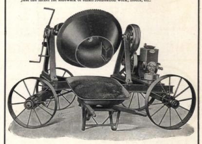
Simplest mixer built. No sharp corners in drum to catch concrete. Convenient side dump. Low charge. Charges or discharges while running at full speed. Mixes wet or dry material equally well. Can be set over sidewalk forms, eliminating wheeling. Equipped with one horse power gasoline engine will turn out more concrete than machines costing twice or three times as much. Can be operated by hand.
