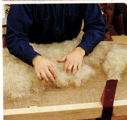
TOP (left to right): To hold the white cowtail hair firmly in place for the roll edging, it is stuffed under slightly loose loops of stitching. The extra flap of burlap is rolled over and then stitched and tacked down to create a well-shaped edge. BOTTOM (left to right): Loops of twine, stitched on all four sides, secure a heavy layer of hair that is worked across the entire piece. After there is a solid base of hair, more burlap is attached to pull the hair down flat.
