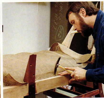
TOP (left to right): To hold the white cowtail hair firmly in place for the roll edging, it is stuffed under slightly loose loops of stitching. The extra flap of burlap is rolled over and then stitched and tacked down to create a well-shaped edge. BOTTOM (left to right): Loops of twine, stitched on all four sides, secure a heavy layer of hair that is worked across the entire piece. After there is a solid base of hair, more burlap is attached to pull the hair down flat.
