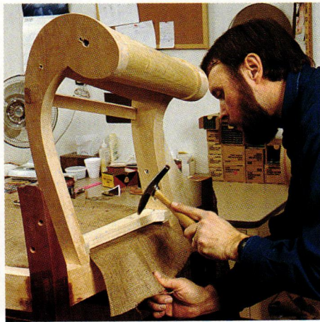
The burlap, which is kept smooth and tight, is tacked at even intervals around the frame. Any excess that isn't needed for a fold is trimmed off.
