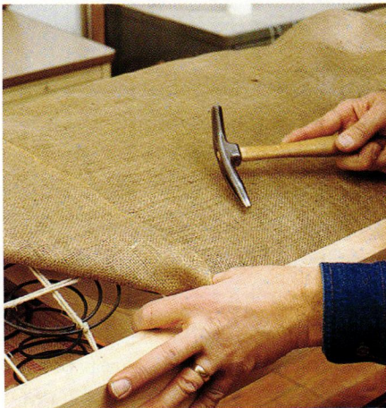
The secured springs are covered with burlap. Since both hands are needed to work with material, upholsterers use a magnetic tack hammer to pick up the tacks.
