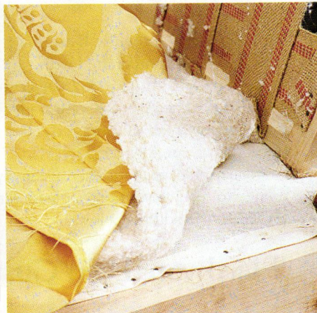
Because the wiry horsehair can poke through the muslin, cotton padding serves as a buffer between the final layers of fabric.
