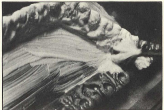
6. First coat of rubber latex is applied carefully so all crevices are filled and no air bubbles remain. Latex, available in art supply stores, cures in about 8 hours—ready for the next coating.
