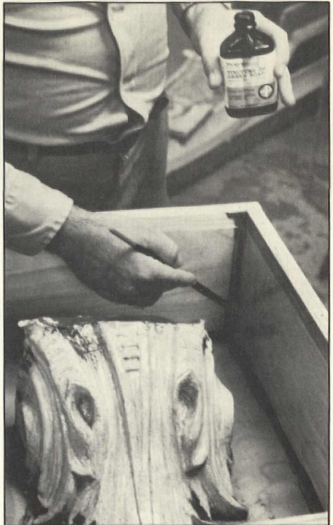
5. Master is given three coats of shellac to seal in impurities left by paint striping. Then coat of green soap is applied so rubber mold will release easily.
