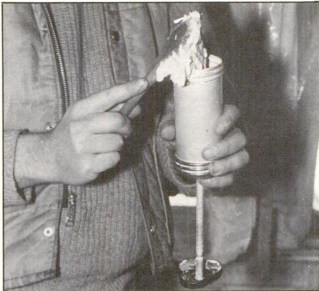
Before loading the compound in the cylinder mix it well to avoid lumps. When the cylinder is full thump it on a hard surface to get out all the air.
