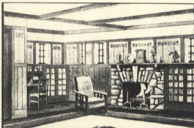
Living room with split boulder fireplace, nook with built-in bookcases and desk, division of wall spaces by wainscoting, stencilled panels and frieze, with casement windows set high in the wall.
