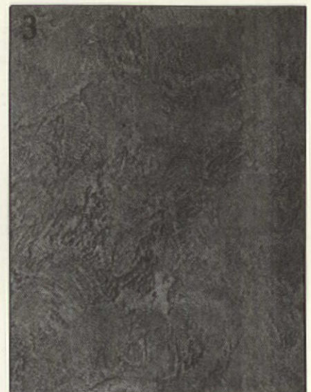
3 ITALIAN PLASTER FINISH -- (Illus. 3) Plaster or texture paint can be used to produce this finish. The material is brushed on with a large paintbrush, then randomly stippled with a stippling brush. After the plaster or paint becomes tacky, brush in random semicircles with a short-bristled paintbrush. As soon as the material has set enough to hold its shape, lightly skim the surface with a plasterer's steel trowel. Glaze topcoats were often used with this finish.
