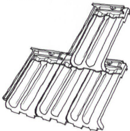
French tile – A large, interlocking shingle tile with deep grooves that give strong shadow lines and channel water.
