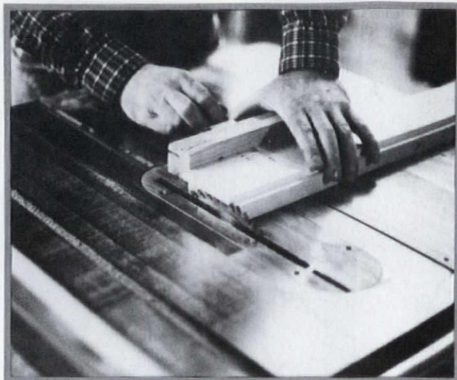
Fig. 2: Cutting the Lap Joint
