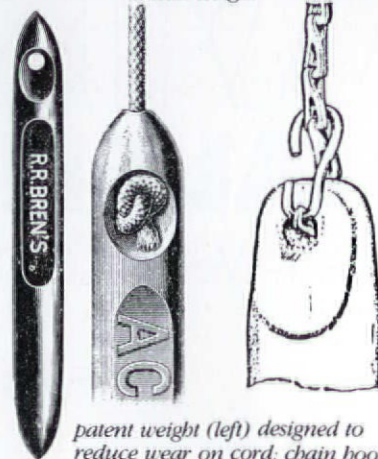
attachment of sash cord to sash weight
