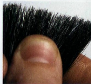
Look for both tapered and flagged bristles (top) by fanning the brush (above).
