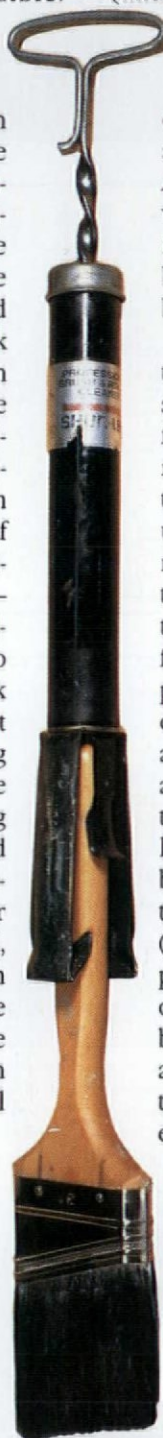
A brush spinner operated by pumping the handle.
