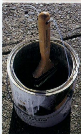
Wrapping in cardboard or paper (top) maintains brush shape during storage. Suspend brushes (above) during any soaking to avoid misshaping the bristles.
