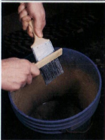
Top: Spinning a brush free of wash wastes. Bottom: Combing is beneficial before and after spinning.
