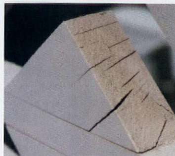
A minor failure, end-grain checks on some diamonds, showed up after a year's exposure.
