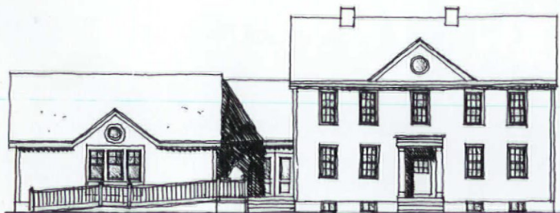
ABOVE: A reduced scale subordinates the proposed annex to this 18th-century Greek Revival house at Williams College. The connecting “hyphen” limits changes to the historic fabric. RIGHT: Setbacks have long been used to subordinate additions. Both main house and extension were built in the 1840s for the daughter of a pea farmer in Mount Carmel, Connecticut. The wing served as a buttery and contained an indoor well.
