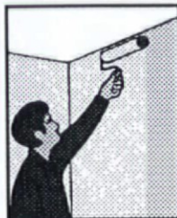
2. Apply saturant to area to be covered.
