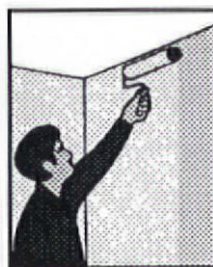
2. Apply saturant to area to be covered.
