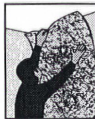
3. Apply fiberglass mat to wet surface.
