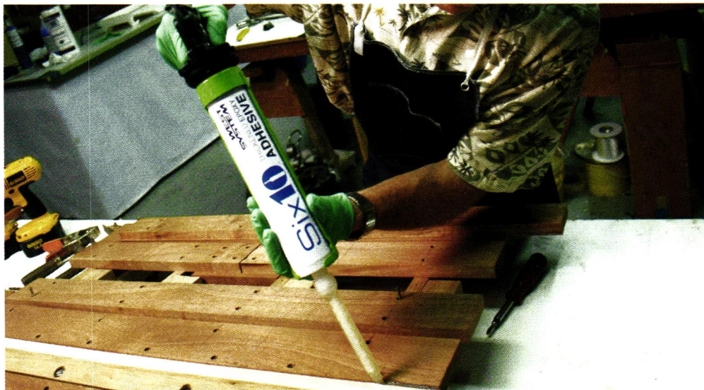
Dispense Six10 Thickened Epoxy Adhesive from any standard caulk gun.
