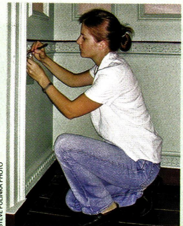
The author excavates small chunks of paint to study cross-sections under a microscope.
