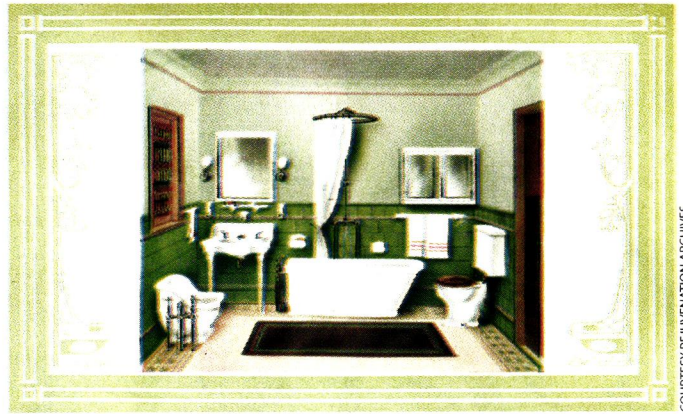
An ordinary-style tub—sloped at the head, flat and plumbed at the foot—was the most common, and affordable, early porcelain model.
