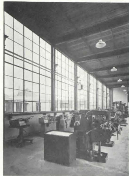
Above — truck entrance (east) end of building. Right — detail of north wall of main hall; continuous bus duct at window-sill height allows attachment to power at any point.
