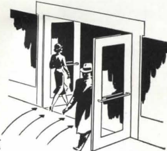
Another spring and hydraulic check controls outswing
