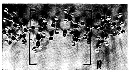
Figure 1—single-molecule chain in cellulose fiber is made up of hexagonal units formed by five carbon atoms and one oxygen atom (above). Each unit contains three hydroxyl groups of one oxygen atom and one hydrogen atom.
