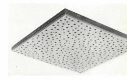
Acoustic Tile: "Full Random"/ nondirectional perforation design in "Cushiontone" fiber tile/ narrow bevel edge/ white-painted surface reflects 78% of light that strikes it/ washable/ available with flame-resistant-paint finish/ 12" squares in  $\frac{1}{2}$ " and  $\frac{3}{4}$ " thickness/ Armstrong Cork Company, Lancaster, Pa.
