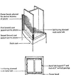
A new method of fireproofing steel columns, developed and tested at the Underwriters' Laboratories, employs lightweight-aggregate plaster and self-furring metal lath bent to fit columns. Indentations in the lath hold it  $\frac{1}{4}$ " from the steel surface, providing space for the plaster to key. No channel furring is required. Metal Lath Manufacturers Assn., Engineers Bldg., Cleveland 14, Ohio.
