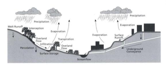
Right: Diagram of natural versus urban hydrology. Courtesy Kerry KenCairn. Opposite page: Diagram of water purification process in Shop Creek, Denver, Colo. Designer: Wenk Associates. Courtesy Kerry KenCairn.
