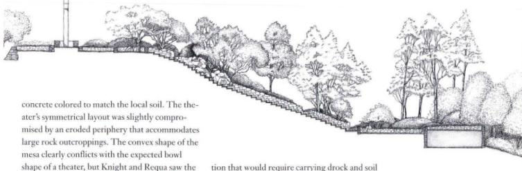
They then looked to the site itself to create a theater form that reflected the topography. The auditorium is long and narrow to minimize the amount of fill required to counter the conical shape of the mesa. The most unique adaptation is the way the aisles and central seating rise above the side sections to reflect the site's convexity, creating modulated shadow patterns along the stepped aisles:
