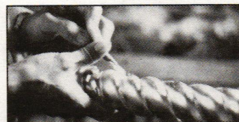
Gold Leaf Studios craftsman gilding a rope-twist molding for a reproduction 19th-century mantel mirror.
