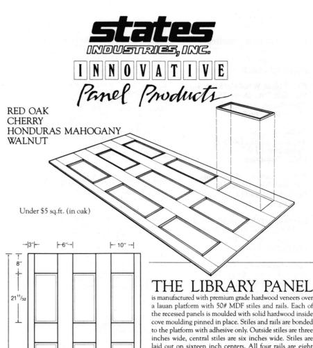
a lauan platform with 50# MDF stiles and rails. Each of the recessed panels is moulded with solid hardwood inside cove moulding pinned in place. Stiles and rails are bonded to the platform with adhesive only. Outside stiles are three inches wide, central stiles are six inches wide. Stiles are laid out on sixteen inch centers. All four rails are eight inches wide.
