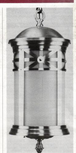
■ Early 20th century turned, spun, and sheet brass lantern with shatterproof plastic. The "Union Jack" decoration can be changed, duplicated at the bottom, or made with three bands. Sizes: Large — 28" O.D., 52" high; Medium — 16" O.D., 28" high; Small — 9" O.D., 19" high. Small unit could use glass for residential installations.
