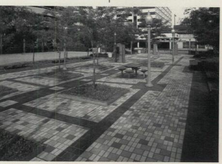
METROPOLITAN CERAMICS supplies paving and flooring materials for both interior and exterior applications. Here, the company's 1/2-in.-thick quarry tiles were used to pave Rotary Park in Canton, Ohio. "Quarrybasics" tiles in three colors at 4-x-8-in. and 8-x-8-in. sizes were used for the light areas, and "Ironrock" flashed color pavers in both sizes were used in the darker areas. Write in No. 54
