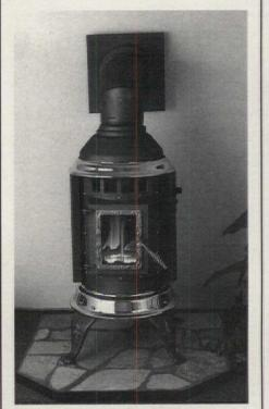
The room-heating Gnome direct-vent gas stove from THELIN has a Turn-of-the-Century potbellied-stove appearance, but uses direct-vent technology with combustion air supplied from outside. It operates with natural gas or propane; another model, the Parlour stove, is a house heater. Both Gnome and Parlour are available in pellet-stove models.
