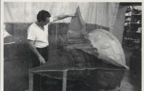
This large rubber blanket mold was made with Poly Latex 80 from POLYTEK DEVELOPMENT CORP. Multiple coats were brushed on a sculpted resin model, allowed to dry, and then peeled off. Write in No. 6360
