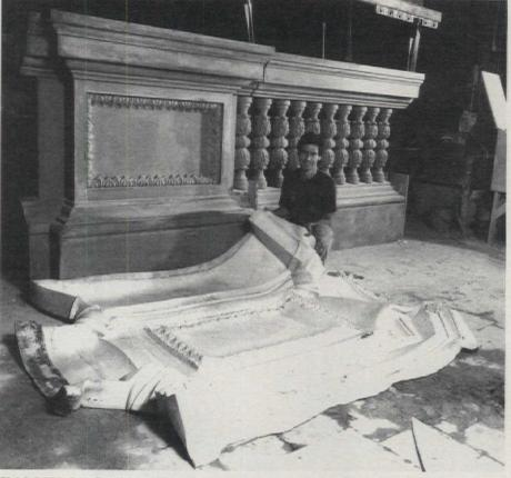
SMOOTH-ON flexible moldmaking materials were used to re-create this oversized wall and balustrade in GFRC. Write in No. 650
