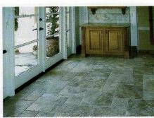
Tumbled travertine from Cantera Especial was used to create this flooring in a Versailles pattern.
