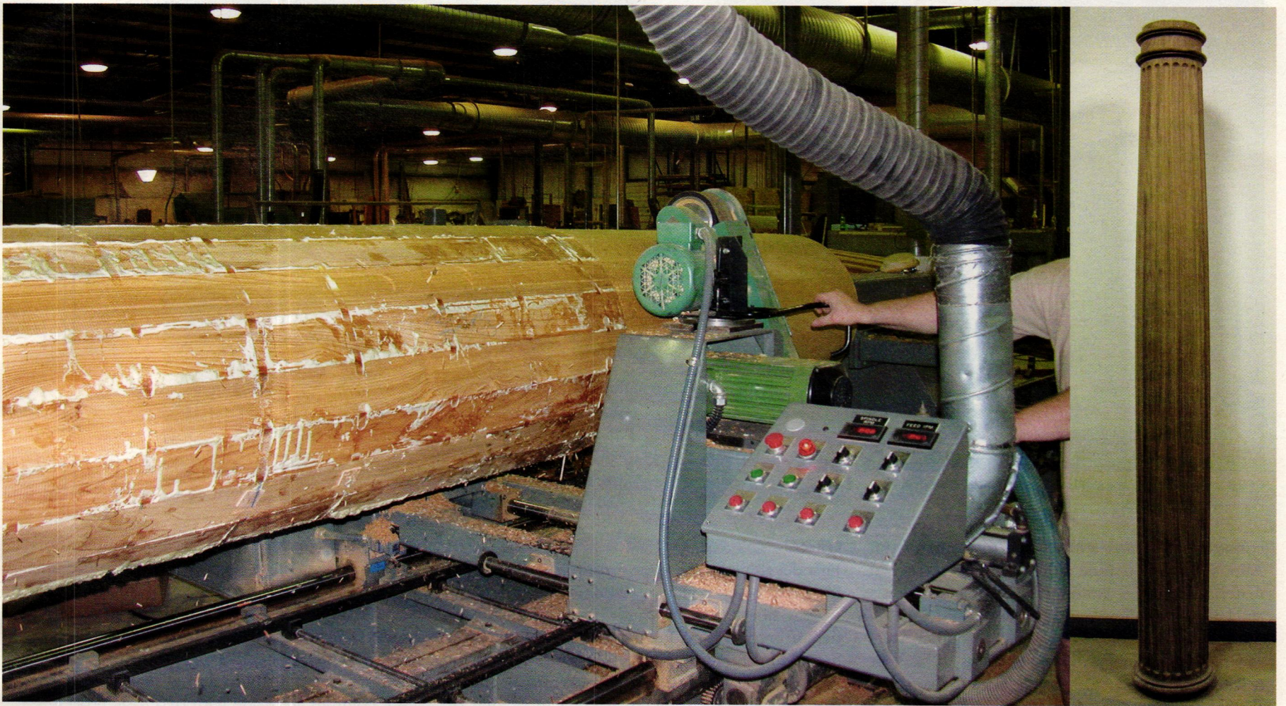
Left: After the column is turned, 24 flutes are cut into the column shaft. The company can manufacture columns up to 40-in. in diameter and 40-ft. long. Right: This walnut Doric column fabricated by Somerset has 24 equal flutes and is ready to be hand sanded. Photos: Somerset Door and Column Co.
