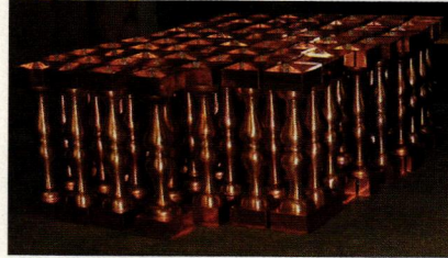
These copper balustrades were fabricated by Heather & Little.
