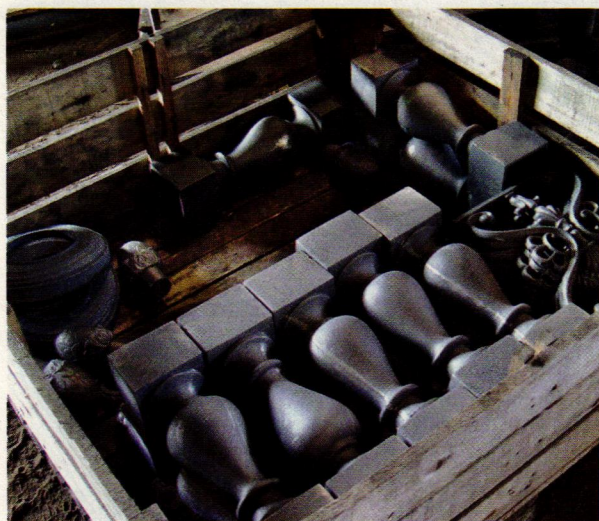
The freshly cast balusters at Robinson Iron's Alabama foundry await shipment to Manhattan. Photo: J. Scott Howell
