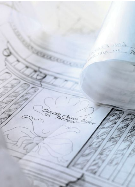
Drawings are enlarged and maquettes are placed on top to verify that the dimensions and proportions of the carving are precise.
