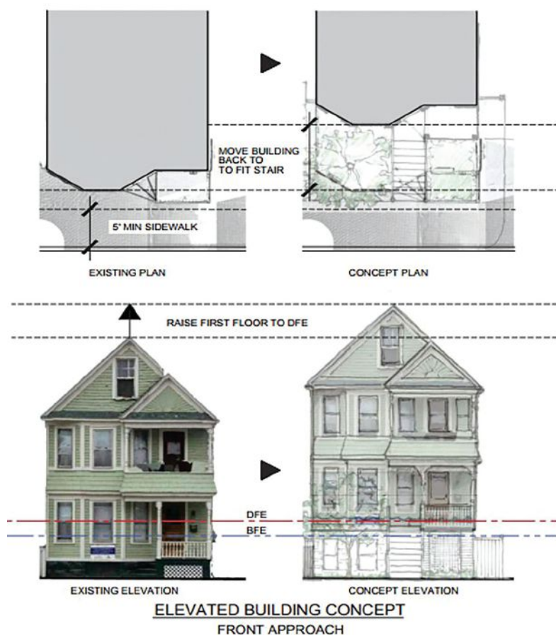
FIG 2 In preparation for the anticipated 44-inch rise in the Chesapeake Bay within the next hundred years, models for community engagement—like this concept for adaptation, raising, and slight relocation of a historic house—helped establish a collective vision for Annapolis. This suite of shared goals, objectives, and community buy-in will shape the city’s climate-change response over the years to come.
